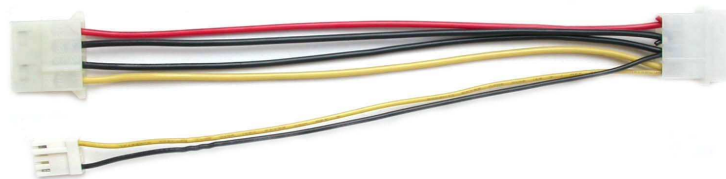
Figure 7: Twelve Volt Power Cable
